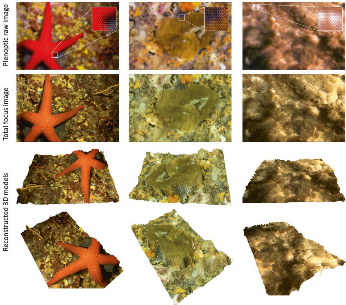
**Fig. 9.11** Underwater images taken using a plenoptic camera (first row), it shows also the repetition of an edge in the scene which is essential to perform the depth estimation. The processed total focus image (second row) and reconstructed 3D models (third row)
