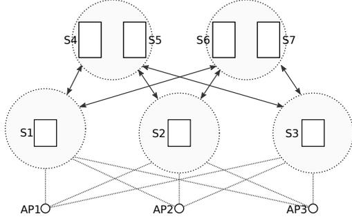
Figure 11: Example of hierarchical topology with 2 layers of clusters.
