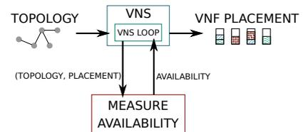
Figure 10: Illustration of our VNS algorithm used as a black box to optimize any NFVI: our VNS receives the description of the NFVI and a methodology to compute the availability of a placement on such an NFVI, producing a VNF placement.
