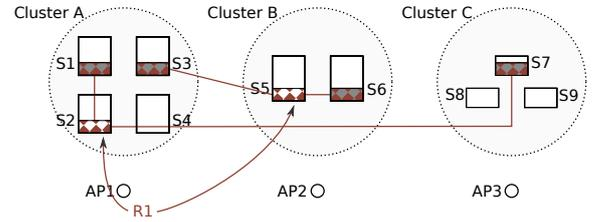
Figure 5: Example of assignment configuration  $\gamma = \{(S2, \{S1, S2, S7\}), (S5, \{S3, S5, S6\})\}$ , where request R1 is split and assigned to two different master VNFs on servers S2 and S5. Both masters have slaves: the master VNF on server S2 has slaves on servers S1 and S7, while the one on server S5 has slaves on servers S3 and S6.
