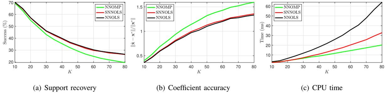
Fig. 2. Average accuracy and CPU time of NNOMP, SNNOLS, NNOLS over 200 trials in a simulated sparse deconvolution problem with Gaussian kernel ( $\sigma = 5$ ). The SNR is set to 18 dB. The dictionary size is  $1200 \times 1170$ .
