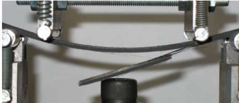
Figure 12: Typical final pattern of co-bonded specimens.
