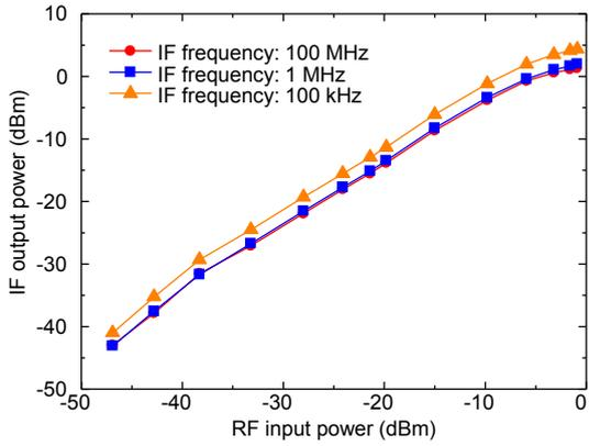
Fig. 5. Measured RF-IF power characteristics of the millimeter-wave receiving front-end module at 76.5 GHz.
