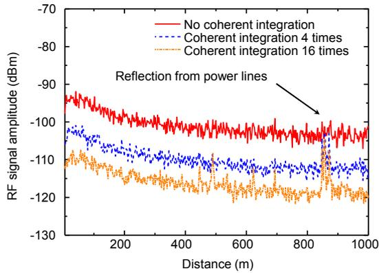
Fig. 10. Example of the measured beat spectrum of the high-voltage power lines obtained with the vertically linear polarized antenna. (Non-coherent integration: 8 times)
