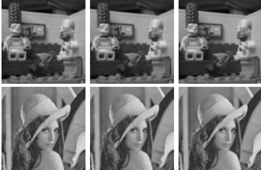
Figure 2: Left: noisy DC image. Middle: denoised DC image ('simpson' PSNR = 40.64 dB , 'lena' PSNR = 40.89 dB). Right: oracle DC image. Top line is the from the simpson image and bottom line from the lena image both with noise of standard deviation \sigma = 30/255 .
