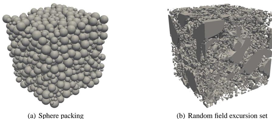
**Figure 1.** *Morphological modelling using non-intersecting spheres packing or random fields.*
