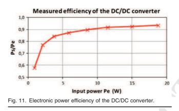
342 converter. The DC/DC converter works at about 343 100 kHz, and the maximum commuted voltage and current are, respectively, 7 V and 3 A, so the noise 344 345 cannot be avoided. The Simulink model was run ten 346 times for each point, and the energy efficiency over 347 the entire cycle was calculated.
