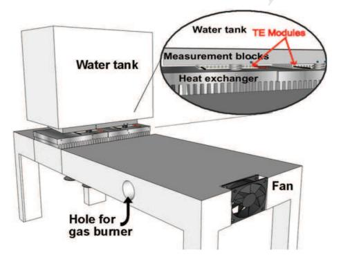
Fig. 14. Test bench for simulating the stove.
