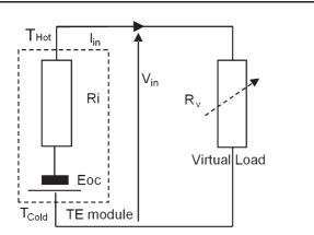
Fig. 5. Electrical model of the TE module and the DC/DC virtual load.
