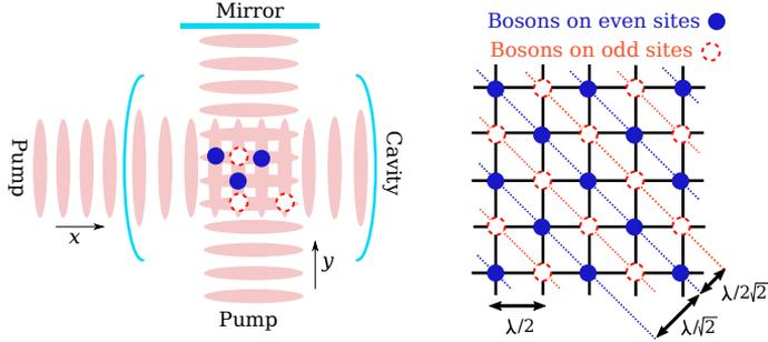
**Fig. 3** (left) In the experiment [17], a 2D gas of cold atoms is subjected to two perpendicular modes in a cavity. (right) The two optical modes are coupled if the atoms adopt a chequerboard pattern that provides the right wave planes to couple modes by scattering.
