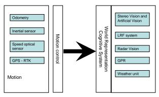
Fig. 1 – simplified sensing architecture of RAS
