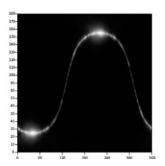
Fig. 4 – Speckle Velocimeter is based on the classical idea of the relative speed calculation starting from regular or quasiregular terrain textures and is developed with the idea of applying a laser-induced speckle pattern to surfaces texture-free like the snow can become. Speed vs Angle plot for a laboratory experimental test of the Speckle Velocimeter
