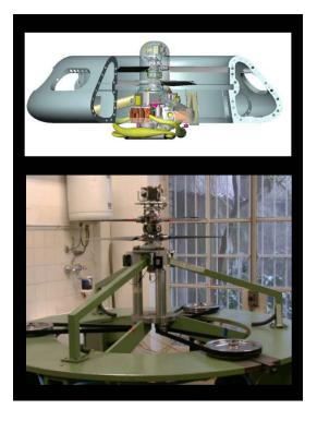
Fig.8 – Preliminary design of the RPV and tests of the propulsion system
