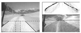
Fig. 3 – Examples of the AV results obtained with the Hough transform algorithm and with ACO (Ant Colony Organisation) algorithm. The result is the detection of the path to follow during a multivehicle raid.
