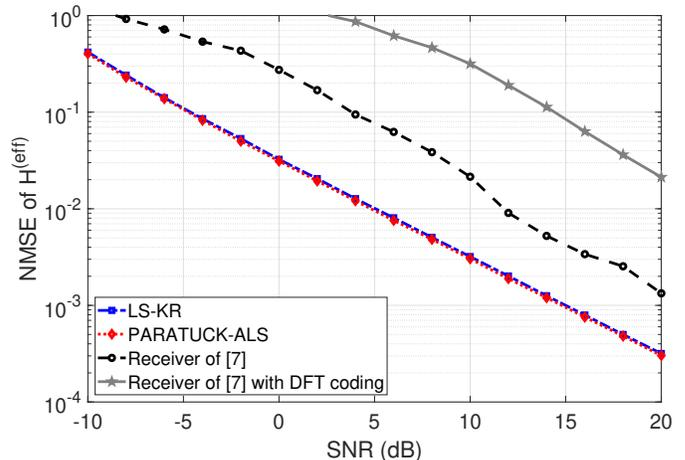
Fig. 10. NMSE versus SNR for the effective channel  $\mathbf{H}^{(eff)}$  for the LS-KR, PARATUCK-ALS receivers and the receiver of [7] using its original Vandermonde matrix coding and the DFT coding used in the proposed receivers.
