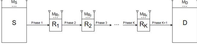
Fig. 2. MIMO cooperative system model with  $K$  relays.
