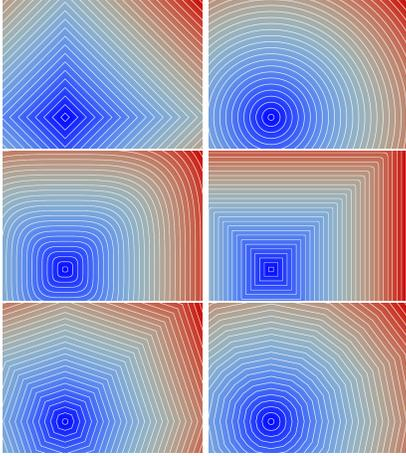
Figure 4: Distance transformation from a single source for different metrics satisfying Definition 4 and thus Proposition 2: (from left to right)  $L_1$ ,  $L_2$ ,  $L_4$ ,  $L_{80}$ ,  $\mathcal{M}_{3-4}$  and  $\mathcal{M}_{5-7-11}$ .
