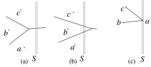
Figure 2: Geometrical predicates for Voronoi map construction Coeurjolly (2014): HIDDENBY( $a, b, c, S$ ) returns true in (a) and false in (b) (straight segments correspond to Voronoi diagram edges). (c) illustrates the CLOSEST( $a, b, c$ ) predicate for  $a \in S$ .
