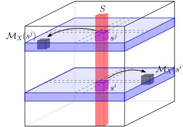
Figure 3: For two points  $s^i$  and  $s^j$  (in purple) on a span  $S$  along dimension  $q$  (in red), the partial Voronoi map images  $\mathcal{M}_X(s^i)$  and  $\mathcal{M}_X(s^j)$  (in black) respectively have  $i$  and  $j$  as  $q^{\text{th}}$  coordinate.
