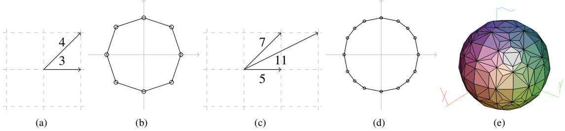
Figure 1: Chamfer masks and rational balls: in dimension 2, generator vectors for the mask  $\mathcal{M}_{3-4}$  (a), its rational ball (b). Generator vectors for  $\mathcal{M}_{5-7-11}$  (c) and its rational ball (d). In dimension 3, rational ball of a chamfer mask obtained using generator vectors  $(x, y, z) \in \llbracket -3, 3 \rrbracket^3$  and weights computed following Fouard and Malandain (2005).
