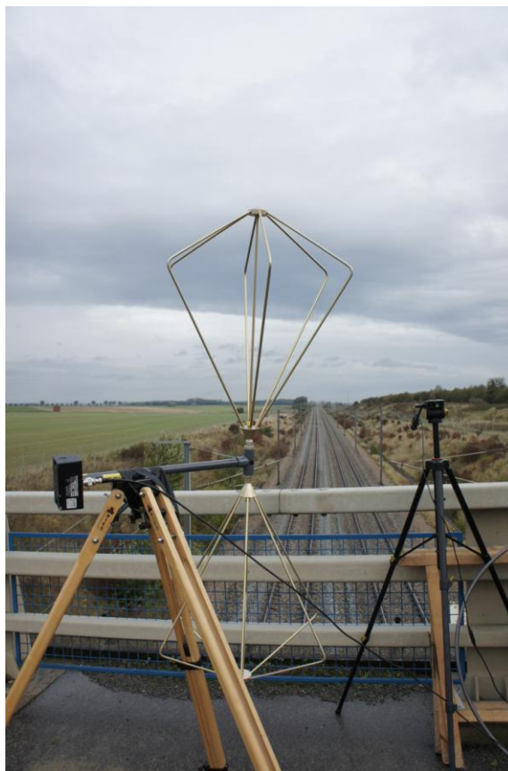
Fig. 2. Measuring antenna location over the railway track.
