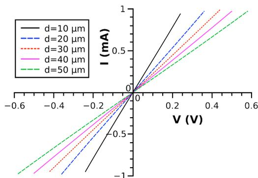
**Fig. 1:** I-V plots as a function of the spacing distance between pads of a typical TLM pattern on non-annealed VLS grown p<sup>+</sup> doped island
