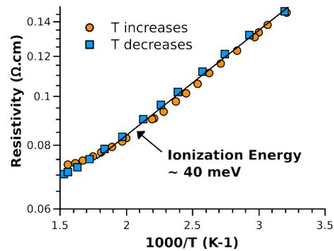
**Fig. 4:** Arrhenius plot of the VLS layer resistivity.
