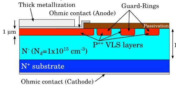
**Fig. 5:** Cross section view of the fabricated diodes.
