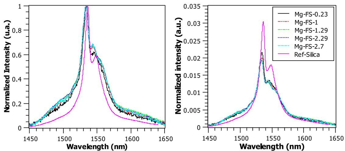
**Figure 5.** Maximum-normalized (on the left) and area-normalized (on the right)  $\text{Er}^{3+}$  emission spectra of magnesium-doped samples. Samples are labeled according to their content in magnesium.
