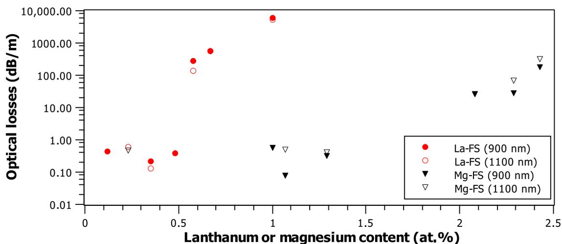
**Figure 4.** Optical losses of lanthanum- and magnesium-doped fiber samples measured at 900 and 1100 nm.
