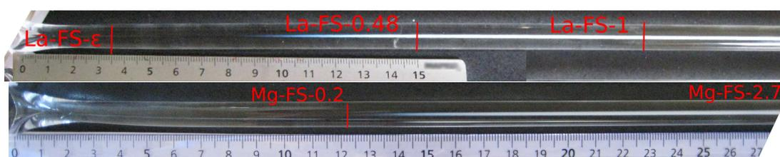
**Figure 1.** Pictures of the La-doped (top) and Mg-doped (bottom) optical preforms. For both preforms, the core whitens with the increase in La or Mg content along the length of the preform. Estimated positions in the preform of the extrema fiber samples are indicated by vertical lines.
