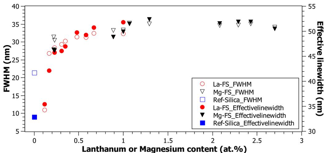
**Figure 9.** Evolution of  $\text{Er}^{3+}$  emission bandwidth with lanthanum (black) and magnesium (red) content. Ref-silica values are shown in blue. Circle symbols are used for the effective linewidth (on the right scale) and crosses are used for FWHM (on the left scale).
