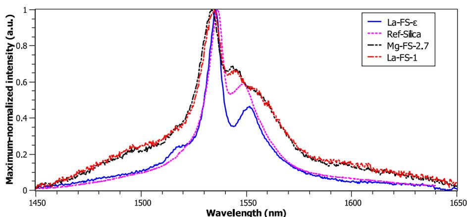
**Figure 7.** Comparison of the maximum normalization of  $\text{Er}^{3+}$  emission spectra of the  $^4\text{I}_{13/2}$  level in fiber samples. Emission spectra of highly doped Mg and La fiber samples are displayed with Ref-silica and low La content samples.
