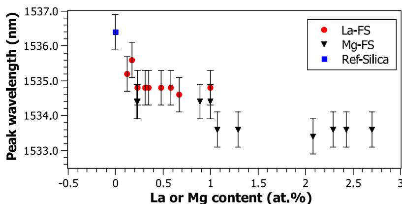
**Figure 8.** Emission peak wavelengths for fiber samples (FS) as a function of magnesium or lanthanum content.
