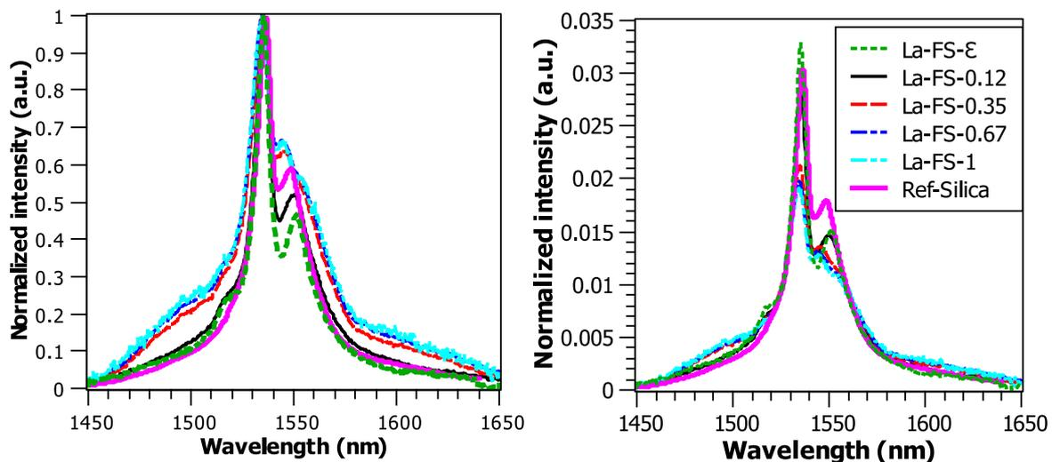
**Figure 6.** Maximum-normalized (on the left) and area-normalized (on the right)  $\text{Er}^{3+}$  emission spectra of lanthanum-doped samples. Samples are labeled according to their content in lanthanum;  $\epsilon$  is used for the sample where lanthanum content was too low to be measurable.
