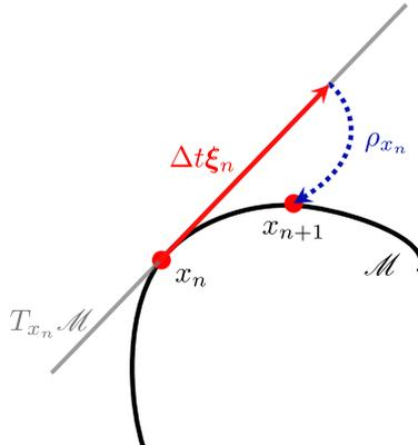
FIGURE 2. Optimization on a manifold  $\mathcal{M}$ : a retraction map  $\rho_{x_n}$  is used to project a tangential motion  $\Delta t \xi_n \in T_{x_n} \mathcal{M}$  from  $x_n \in \mathcal{M}$  back onto the optimization domain  $\mathcal{M}$ .
