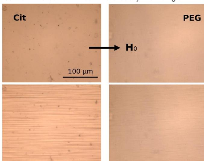
**Figure 1.** Snapshots of aqueous suspensions of citrated (left) and PEGylated (right) MNPs at  $\phi_0=0.13\%$  submitted to  $H_0=13.5 \text{ kA}\cdot\text{m}^{-1}$  at  $t=0$  (upper row) and 5 min after field application (bottom row).
