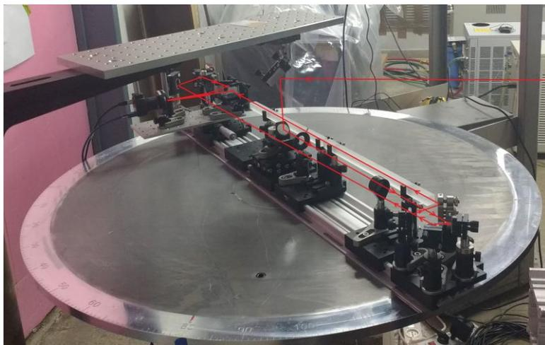
Fig. (1) The Goniometer & Optical Bench. The red line represents the trajectory of the laser pulse with arrows indicating the direction of propagation of the pulse.
