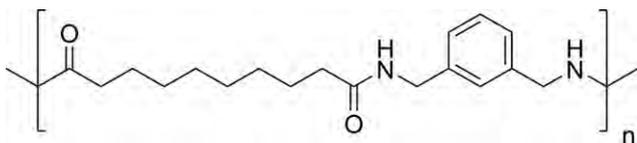
Figure 1. Structure of the PA mXD 10.
