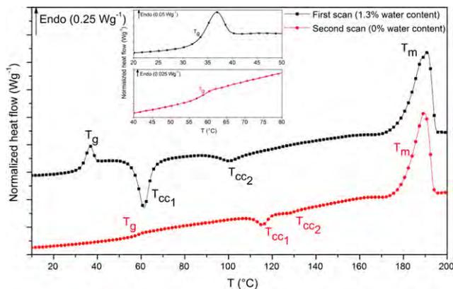
Figure 2. DSC curves of PA mXD 10. A zoom-in of the glass transitions for each heating id reported in the insert. [Color figure can be viewed at [wileyonlinelibrary.com](http://wileyonlinelibrary.com)]
