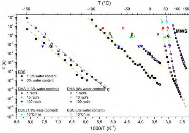
**Figure 5.** Arrhenius plot of relaxation times of PA mXD 10 at 0% and 1.3% water content. (the dashed lines represent the Arrhenius and VFT fits). [Color figure can be viewed at [wileyonlinelibrary.com](http://wileyonlinelibrary.com)]
