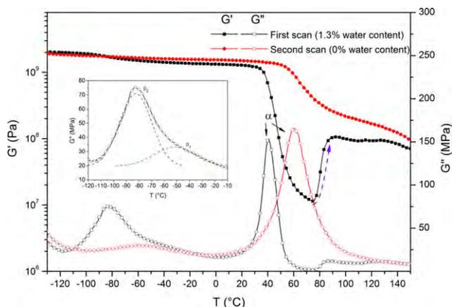
**Figure 3.** First and second DMA scans of PA mXD 10 at 1 rad s<sup>-1</sup>. The filled symbols represent the storage modulus  $G'$  and the empty symbols the loss modulus  $G''$ . A zoom-in of the  $\beta_1$  and  $\beta_2$  relaxations is reported in the insert. [Color figure can be viewed at [wileyonlinelibrary.com](http://wileyonlinelibrary.com)]
