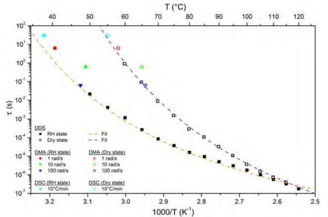
**Figure 6.** Arrhenius diagram of the  $\alpha$  relaxation times and VFT fits (the dashed lines represent the VFT fits). [Color figure can be viewed at [wileyonlinelibrary.com](http://wileyonlinelibrary.com)]
