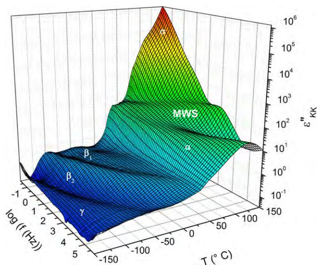
**Figure 4.** 3D spectrum of dielectric loss versus frequency and temperature after Kramers-Kronig transform at 1.3% water content. [Color figure can be viewed at [wileyonlinelibrary.com](http://wileyonlinelibrary.com)]
