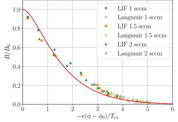
Figure 9: Normalized electric potential with the characteristic estimated  $T_{e^*}$  and comparison with analytical model (red).
