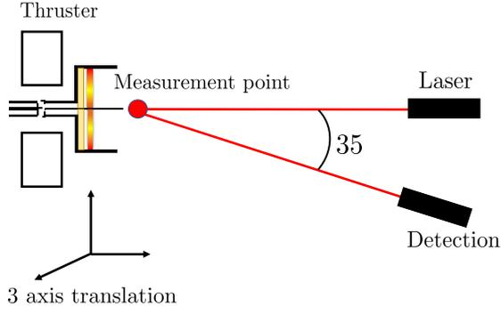
Figure 2: Schematic of optical LIF setup inside the vacuum chamber
