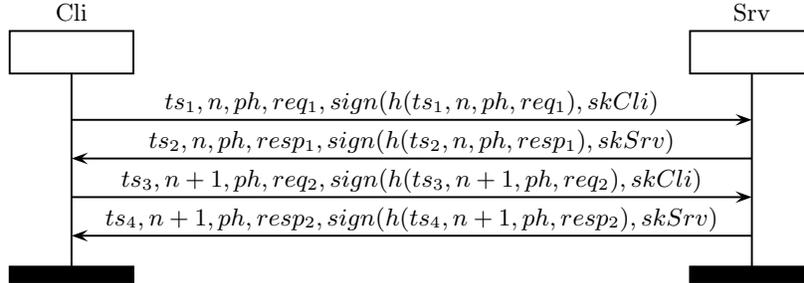
Figure 3: Two requests and responses in secure MODBUS [16].
