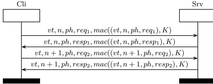
Figure 4: Two requests and responses in secure MODBUS [17].
