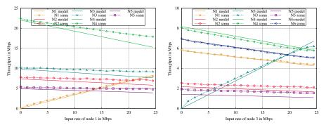
(a) Five-node star, varying the input rate (b) Six-node mesh, varying the input rate of node 1,  $x_1$ . of node 3,  $x_3$ .
