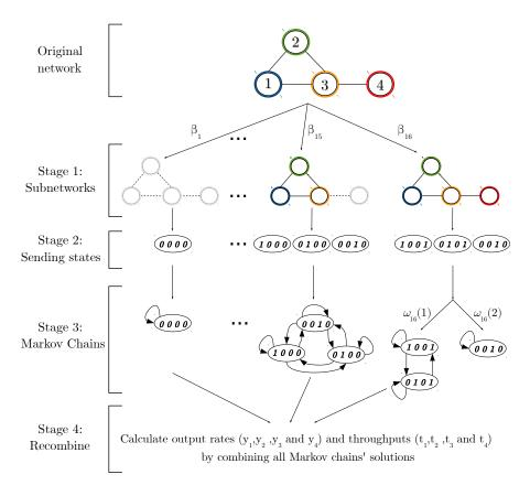
Figure 3: Schematic representation of the proposed solution.
