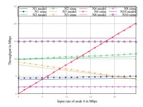
Figure 10: Ten-node network: varying the input rate of node 4,  $x_4$ .
