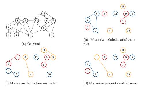
Figure 13: Different channel allocations for a randomly-generated 12-node network.
