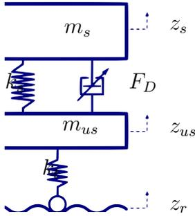
Fig. 1. Semi-Active Quarter of Vehicle model.
