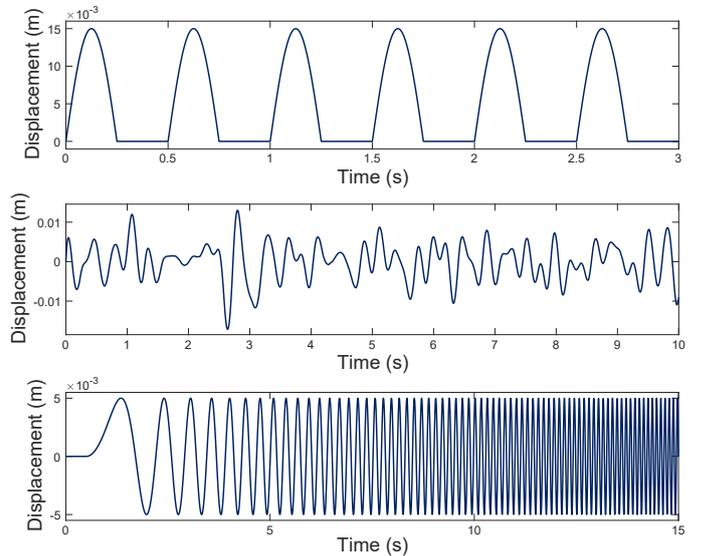
Fig. 5. Road profiles used for simulation tests. Road with bumps (top), Rough road (middle), Chirp (bottom)
