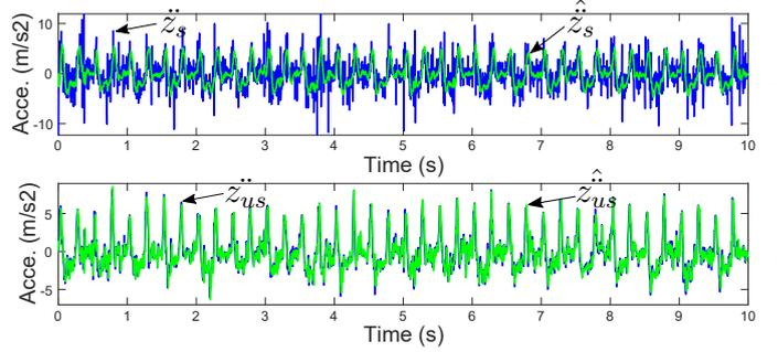
Fig. 9. Sprung and unsprung mass accelerations in test 1.
