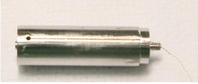
FIG. 5: Modified batch cell of a Setaram microDSCIII calorimeter. The connecting wires get out by a small hole and they are glued inside a thin groove machined along the side of the cell.
