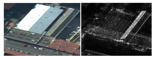
Figure 1: Example of building roof opaque in visible light (left) but transparent at X-band (right). White roofed building hosts a supermarket the aisles of which can be discerned at X-band.
