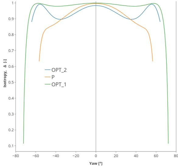
Fig. 9: Isotropy variation along yaw direction ( $I = 80^\circ$ )
