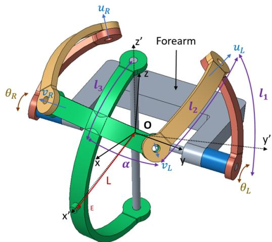
Fig. 1: CAD model of the investigated 2DSPM
