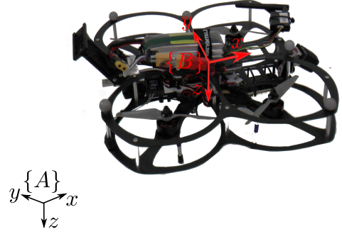
Fig. 1. Quadrotor platform: The platform used for the indoor experiments showing the body-fixed \{B\} and inertial \{A\} frames.
