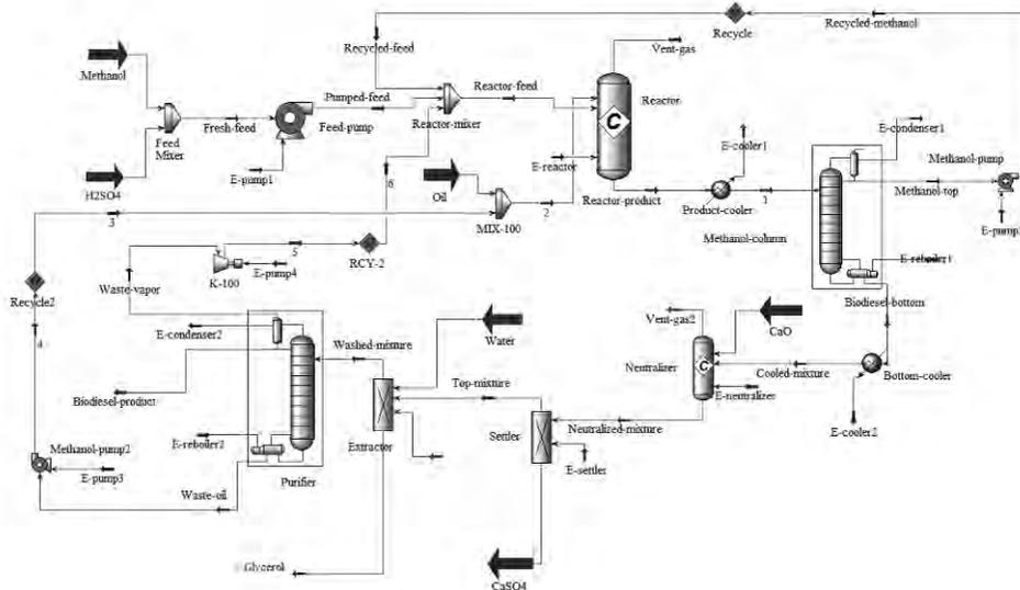
Figure 1. Flowsheet of the acid-catalyzed process obtained with Hysys
