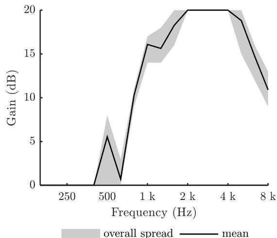
Figure 7: Dispersion and average of the optimal equalisation values of a speech-shaped noise signal by optimisation of the SII obtained from the 11 hearing loss profiles.
