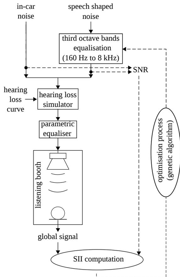
Figure 1: Search procedure for speech signal equalisation in an in-car noise by optimisation of the SII with hearing losses taken into account.
