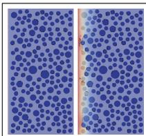
**Fracture of heterogeneous media** : Using a Frictional Cohesive Zone Model or eigen-erosion method, fracture can be modeled, at microscopic or mesoscopic scale, from initiation to post-failure. Recent developments permits to take into account effects of the thermal solicitations.
