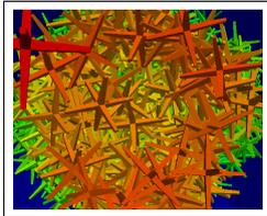
**Granular Material, from rheology to structure** : a typical use of LMG90 concerns the study of the rheology of granular materials. As an example the figure shows a sample made of the deposit of non-convex rigid bodies.
