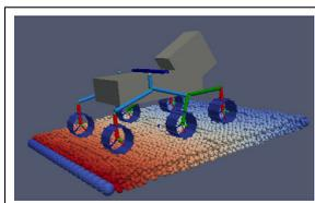
**Coupling with Multi-Body-System** : simulations with software such as Robotran to correctly simulate the behavior of controlled complex systems in interaction with a large number of particles are also possible.
