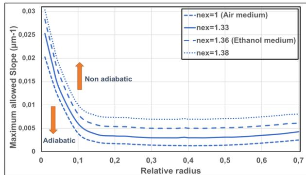
Fig. 2. Adiabaticity limit for different external indices
