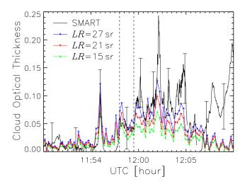
**Fig. 11.** Time series of cloud optical thickness determined from SMART-Albedometer measurements (black line) and from lidar data for different values of the lidar ratio (27, 21 and 15 sr, colored lines). The error bars at exemplary time steps display the uncertainty of the albedometer retrieval. The vertical bars indicate the time interval over which the measured and simulated values were averaged for the spectra shown in Fig. 10.
