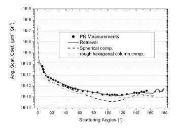
**Fig. 9.** Retrieved angular scattering coefficients at the Polar Nephelometer nominal wavelength (800 nm). Contributions of both components (ice spheres and ice columns) on the cloud total scattering properties are also displayed.
