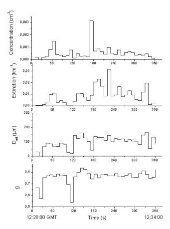
**Fig. 7.** Time series of the concentration, extinction coefficient, effective diameter  $D_{eff}$ , and asymmetry parameter g retrieved from the polar nephelometer.
