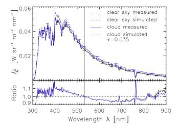
Fig. 10. Top: Spectral downwelling radiance  $I_{\lambda}^{\downarrow}$  simulated (dashed lines) and measured (solid lines) by the SMART-Albedometer for clear sky conditions (black lines) and the observed optically thin midlevel ice cloud (blue lines). The measured and simulated data of the thin cloud are averaged over two minutes (indicated by vertical lines in the time series of Fig. 11). Bottom: Ratio between simulated and measured downwelling radiance for the clear sky and cloudy case.
