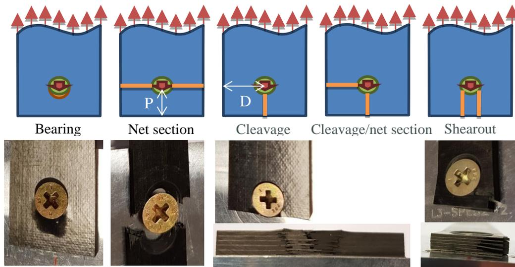
Figure 2. Failure modes of composite bolted joints
