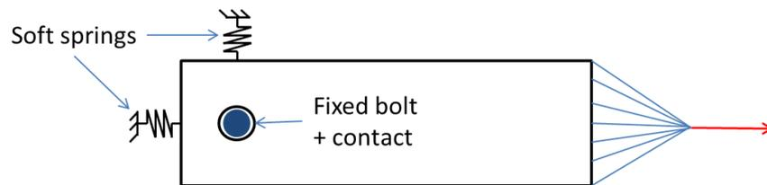
**Figure 7.** Boundary conditions of the 2D FE model
