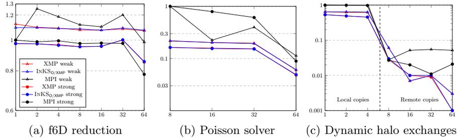
Fig. 3: Weak and strong scaling for 3 parts of the Vlasov-Poisson solver up to 64 nodes (1 process/node) on a  $32^6$  grid divided among processes (strong scaling) or  $16^6$  grid per process (weak scaling). Median of 10 executions.
