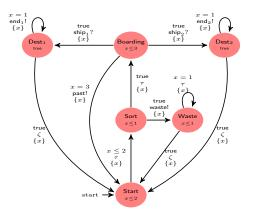
Fig. 1. A conveyor belt specification.
