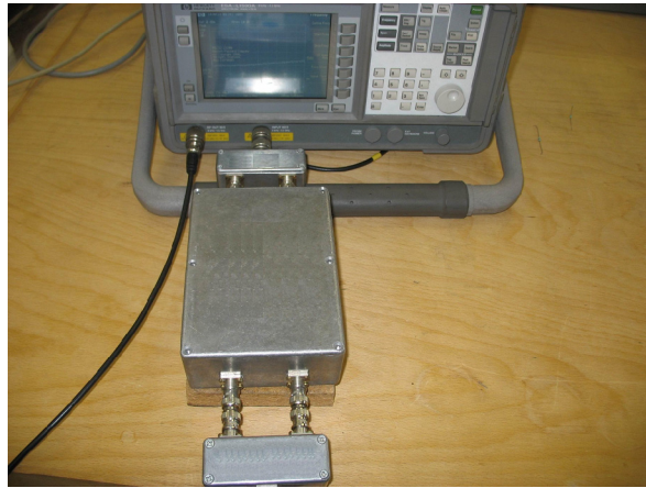
Fig. 14. EMI filter characterization
