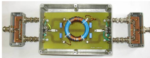
Fig. 15. Experimental EMI filter characterization for CM
