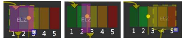
Figure 12: the gauge value is detected by an enter/leave zone
