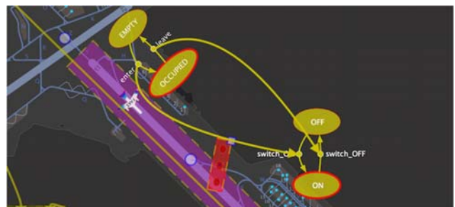
Figure 8: coupling state-machines: here, runway and stop bar
