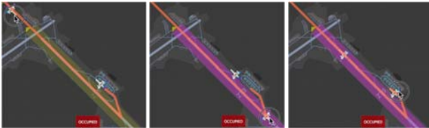
Figure 19: Assessing automation behavior in the near future: pressing on the top-left flight displays its predicted route (in orange), moving the flight along its route changes the time of the whole simulation.
