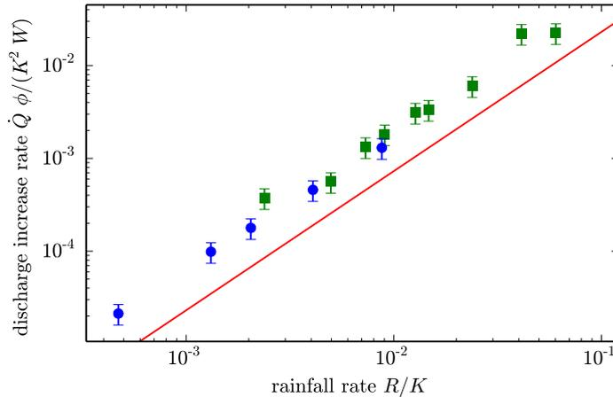
FIGURE 5. Dependence of the discharge increase rate with respect to the rainfall rate, for two series of experiments: 4 mm glass beads (blue dots) and 1 mm glass beads (green squares). The red line represents the asymptotic regime (5.6).
