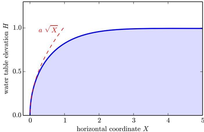
FIGURE 4. Numerical solution of equation (5.2), corresponding to the self-affine shape of the water table during the early stage of a rain event (blue line). Its behaviour near the aquifer outlet is  $a\sqrt{X}$  (red dashed line).
