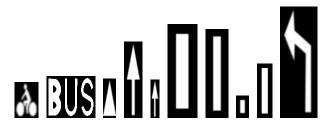
Fig. 3. Library of road marking template patterns (GSD=2cm).
