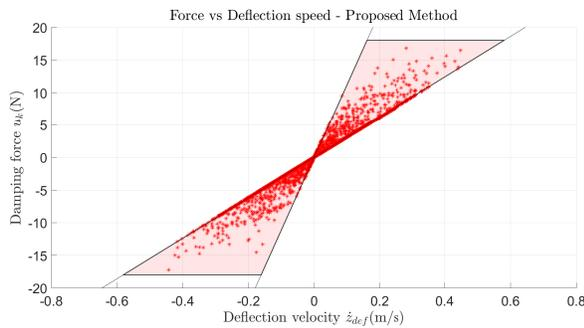
Fig. 4. Damping force vs Deflection speed - Proposed method
