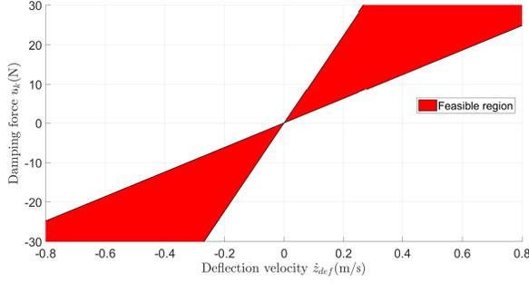
Fig. 2. Damper force vs deflection velocity plot
