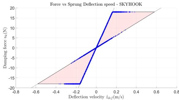
Fig. 5. Damping force vs Deflection speed - Skyhook
