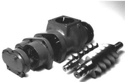
Figure 1. Typical example of oil injected screw compressor
