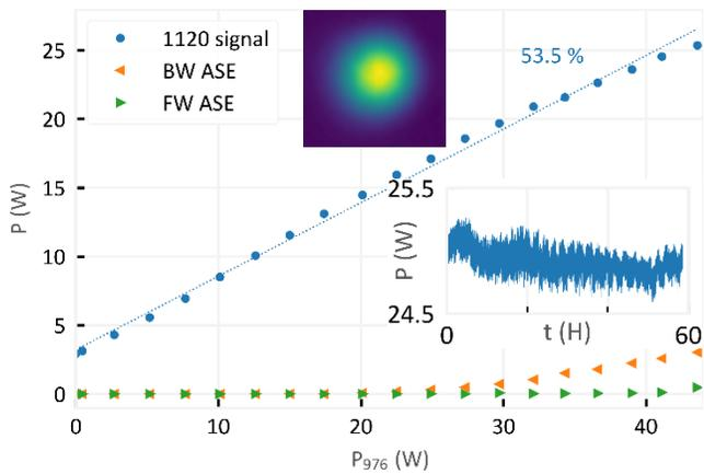
Fig. 2: Output signal and ASE power vs. launched pump power. Insets show mode profile and power stability over 60 hours
