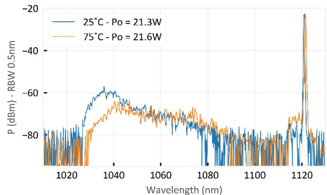
Fig. 4: Effect of heating on output spectrum ( $P_{\text{pump}}=35$  W).
