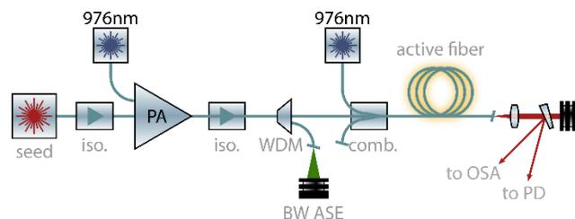
Fig. 1: Schematic of the all-fiber MOPA. Iso.: isolator; PA: Pre-amplifier; WDM: Wavelength-division multiplexer; comb.: Pump combiner; OSA: Optical Spectrum Analyzer; PD: Photodiode; BW ASE: Backward-propagating Amplified Spontaneous Emission
