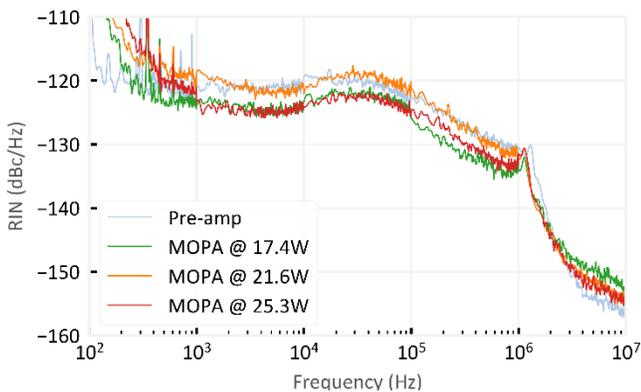
Fig. 5: Measured RINs of the preamp and MOPA for different output powers (detected optical power 10 mW).
