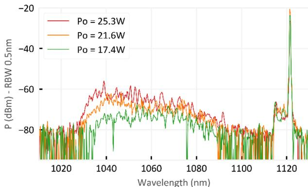
Fig. 3: Output signal spectrum for different output powers.
