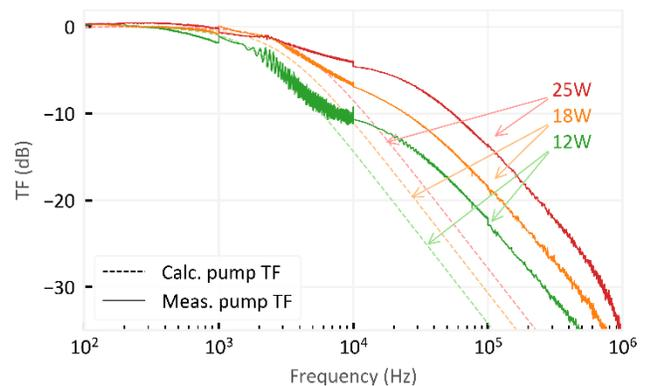
Fig. 6: Calculated and measured transfer functions for pump modulation.
