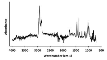
Figure 6 ATR-FTIR spectrum of PP-based coating.
