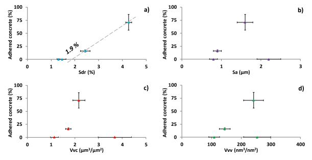
Figure 8: Adhered concrete percentage as a function of: a)  $S_{dr}$ , b)  $S_{a}$ , c)  $V_{vc}$  and d)  $V_{vv}$ .
