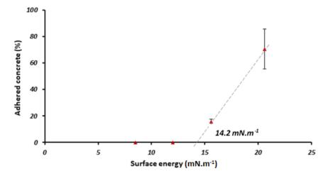
Figure 9 shows the percentage of concrete adhered against the formwork skins as a function of surface energy. Total surface energy and thermodynamic work of adhesion have been proven correlated [55] in agreement with Figure 9. The curve indicated a threshold surface energy of 14.2  $mN \cdot m^{-1}$  below which concrete has minimal surface adhesion with the formwork surface.
