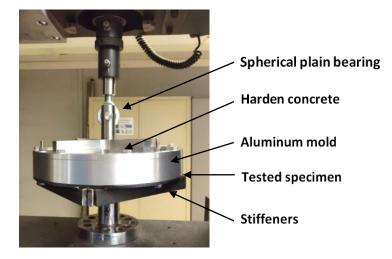
Figure 2 Overview of pull-off adherence test.
