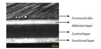
Figure 5 Optical micrograph of the coating put on the formwork skin.
