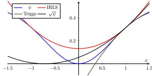
**Fig. 1.** Quadratic surrogate models used by direct approaches at  $\bar{\theta} = 1$  (the x-axis corresponds to  $\theta = \bar{\theta} + \Delta\theta$ ): IRLS (Eq. 3), second order expansion used in the Triggs correction (Eq. 4) (which is concave at  $\bar{\theta}$ ) and “Square-rooting  $\psi$ ” (Eq. 5). Observe that only the IRLS model preserves the symmetry of  $\psi$  and has its minimum at the zero residual.
