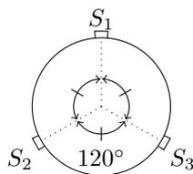
**Figure 1:** Three strain sensors  $S_1, S_2, S_3$  placed on a circular section of a needle with a  $120^\circ$  angle between them.
