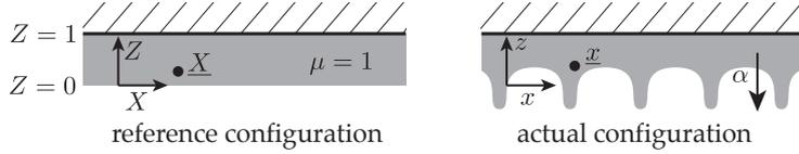
Figure 3: Reference and actual configurations of the elastic slab. We use dimensionless units, with a scaled thickness  $h = 1$ , a scaled shear modulus  $\mu = 1$ , and a scaled weight  $\alpha$  defined in (8). These drawings are shown in 2 dimensions for the sake of legibility; the analysis, however, is done in 3 dimensions: the direction  $Y$  transverse to the plane of the figure is accounted for.
