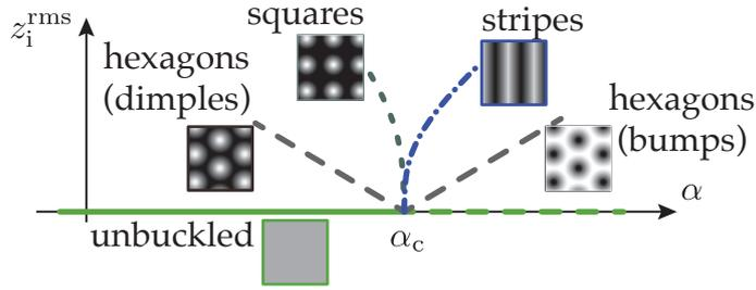
Figure 5: Sketch of the bifurcation diagram in the neighborhood of the bifurcation point  $\alpha_c$ , as obtained by the weakly non-linear analysis, see §5 and §6. Only the part of the unbuckled pattern below the first critical load ( $\alpha < \alpha_c$ ) is stable (solid line). All the other branches are unstable (dashed/dotted curves). An *unsigned* buckling amplitude is used on the vertical axis, which makes the hexagonal branch appear as a broken line.
