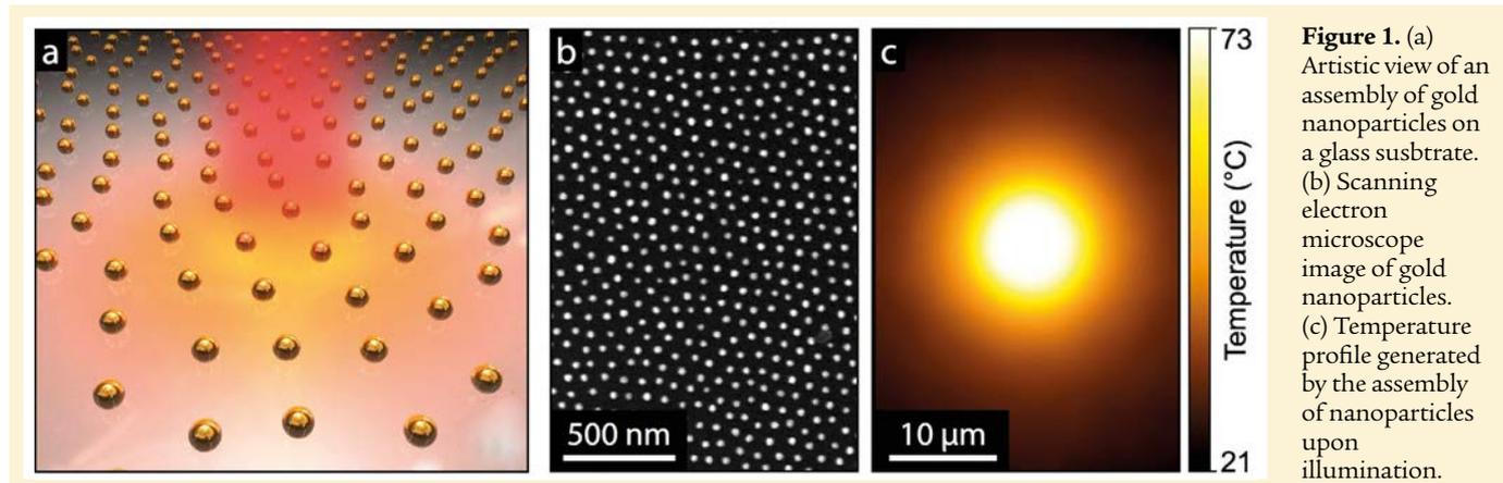
**Figure 1.** (a) Artistic view of an assembly of gold nanoparticles on a glass substrate. (b) Scanning electron microscope image of gold nanoparticles. (c) Temperature profile generated by the assembly of nanoparticles upon illumination.
