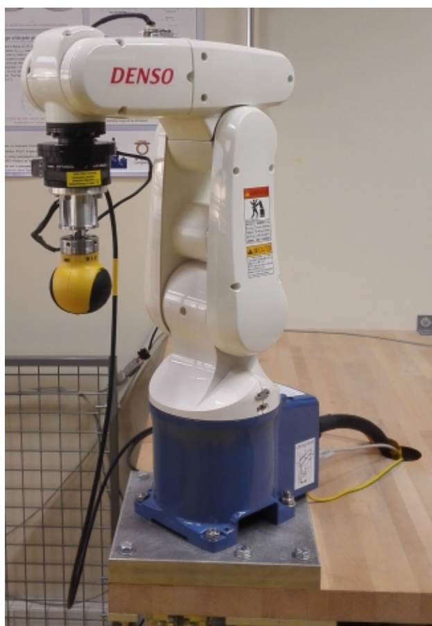
Figure 1: VP-6242G Denso robot.
