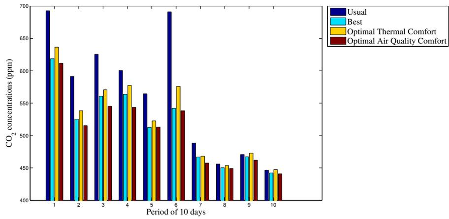
**Fig. 4.** Variation in Indoor CO<sub>2</sub> Concentrations Resulting from Different Schedules in the Experimental Duration.
