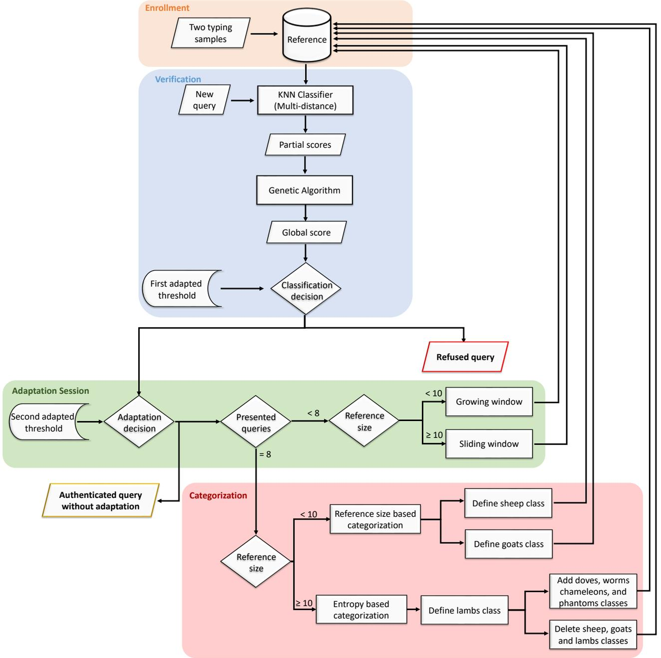
Figure 2: Description of the keystroke authentication process
